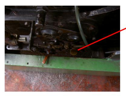
Left gearbox filler point SAE90 HP gear oil. about halfway up tube
